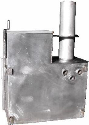
The Hot Tub is heated by an all stainless steel, efficient, wood burning **Aquafire™** stove, which can heat the water to a pleasant soaking temperature in just 2 hours. The stainless steel stove is completed with a UL listed "Selkirk" stainless steel insulated chimney to protect against accidental contact, and a stainless-steel rain cap with spark arrester.
